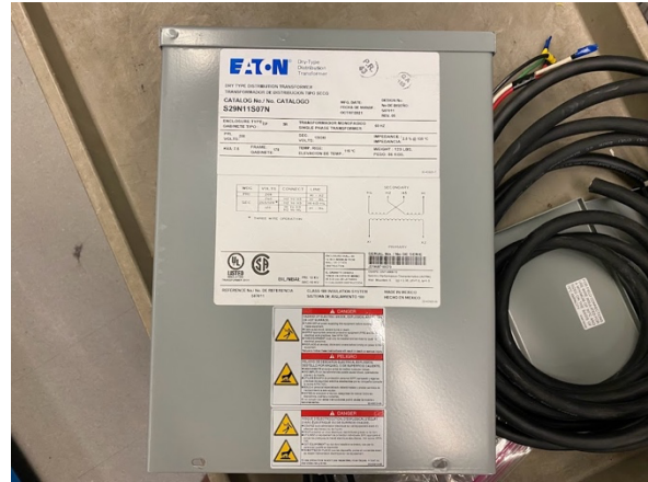
Figure 2: 208/240 V split-phase transformer provided by Eaton.
