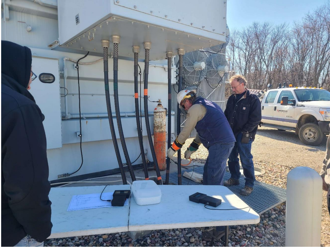
Figure 24: Live field testing on secondary transformer
