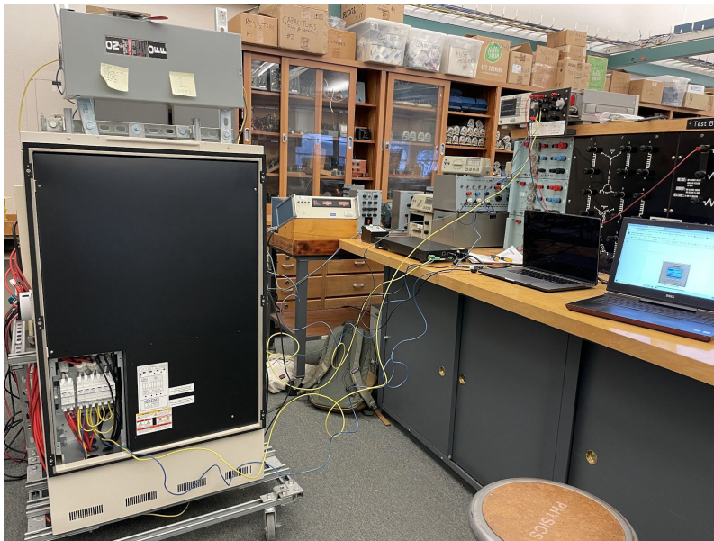
Figure 24: Interfacing of Tabuchi BESS, ITECH Power Supply, and Lab Bench
