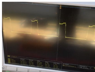
Fig. 18 - Duty Cycle displayed using oscilloscope
