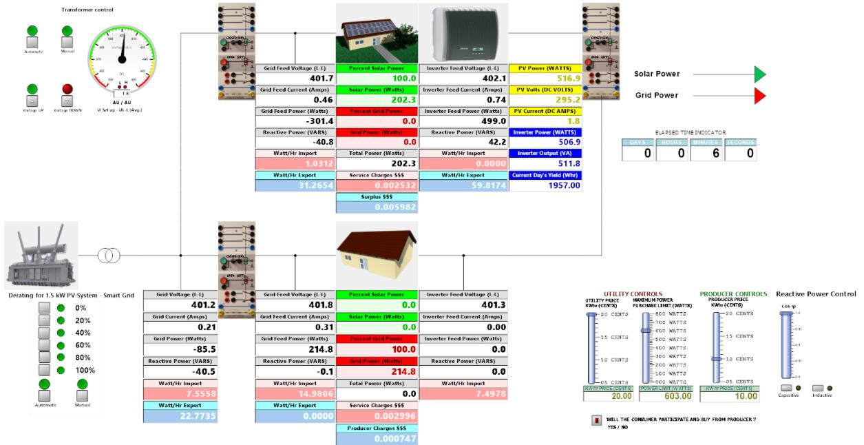
Figure 3. Solar Microgrid SCADA / HMI with Transactive Energy Controls
