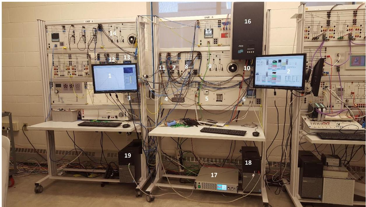
Figure 4. Layout of Photovoltaic/Transactive Energy Component of the Test Bed
