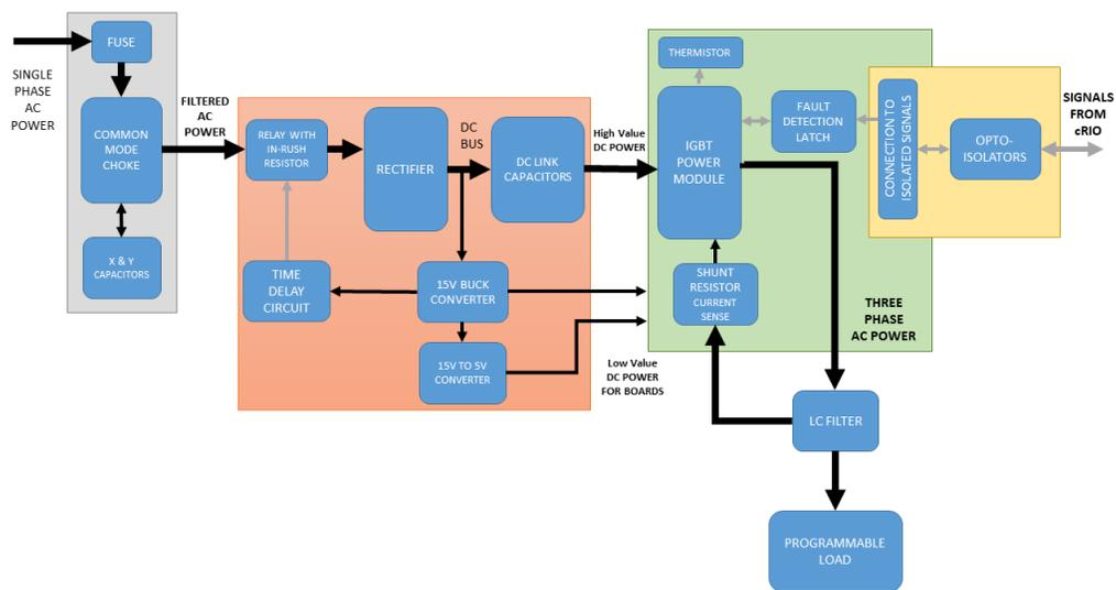
Figure 3: Inverter Block Diagram
