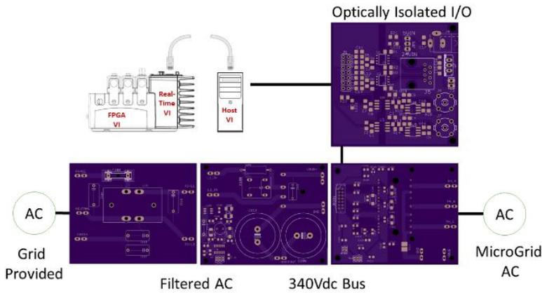
Figure 4: Inverter Board Layout
