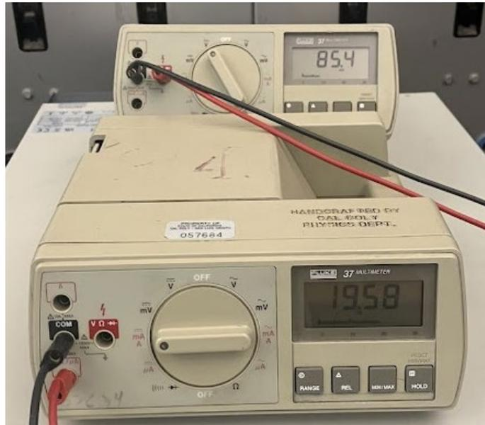
*Figure 18: Voltage reading across battery-2 and current reading through the resistive load when battery-2 is connected to the load.*
