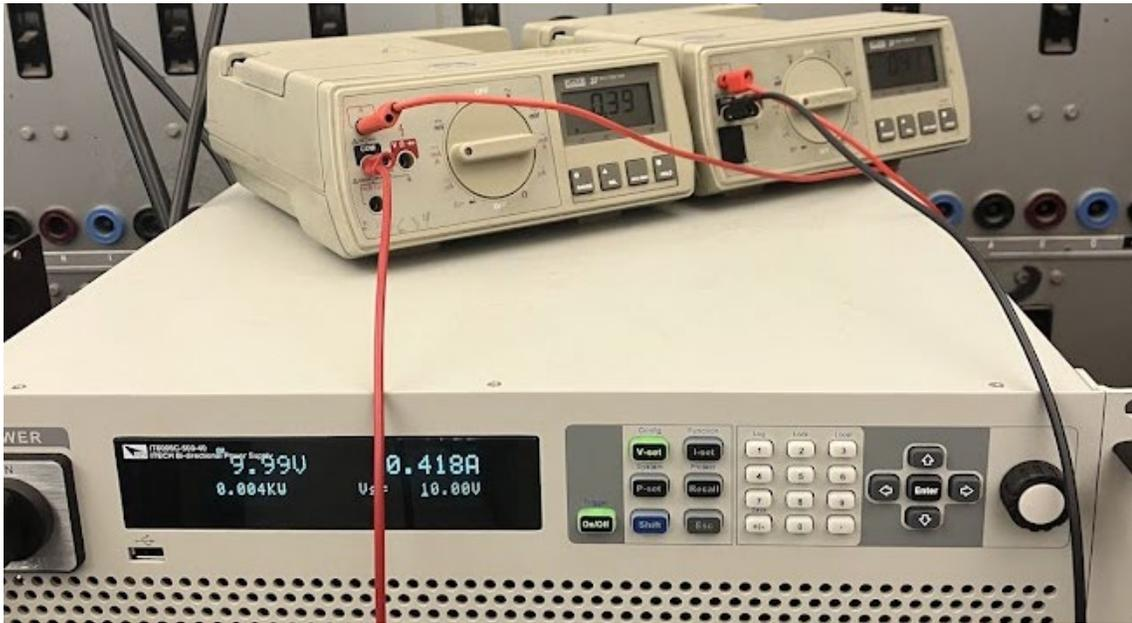
Figure 21:10-Volt test. Ammeter and source current readings: The current drops by  $\frac{1}{2}$  as expected.
