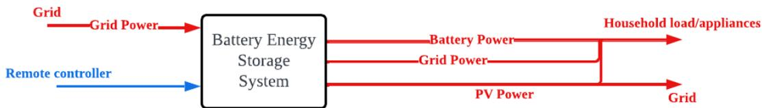
Figure 2:Level 0 Functional Decomposition
