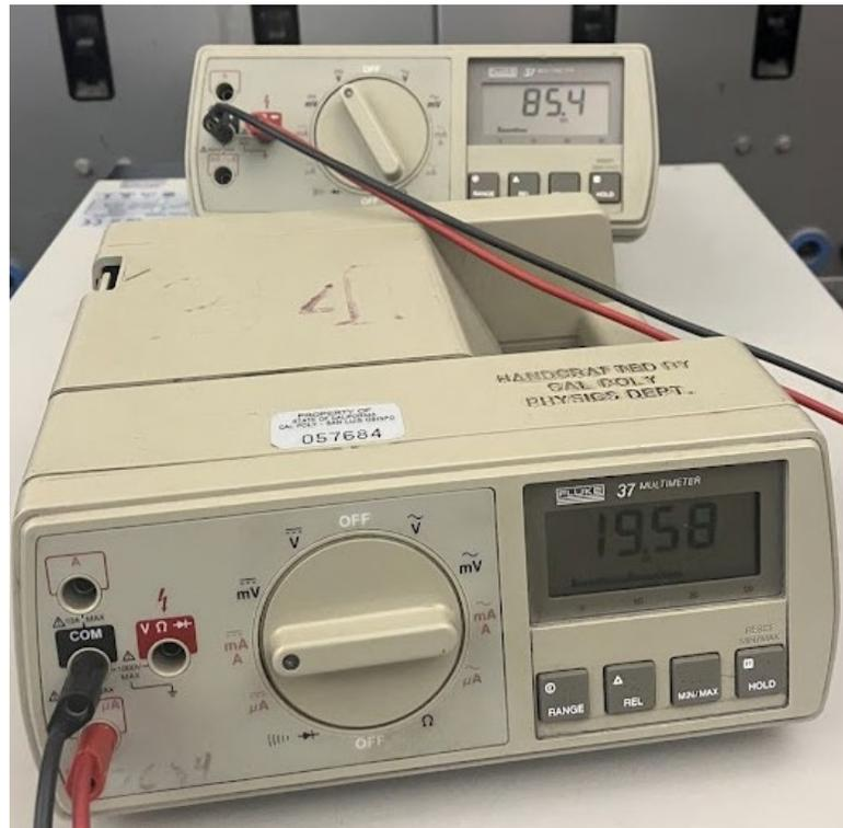
Figure 17: Voltage reading across battery 1 and current reading through the resistor when battery 1 is connected to the resistive load.
