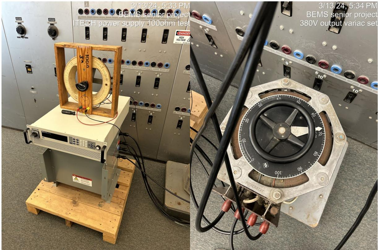
Figure 9: ITECH output test and Variac 380V output setting
