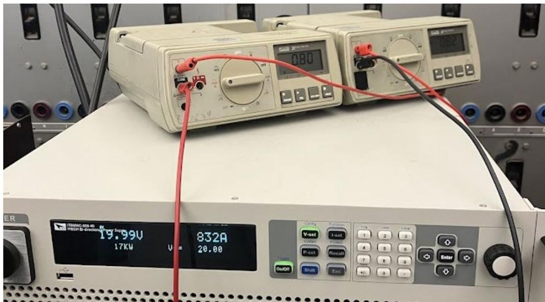
Figure 20: 20-Volt test. The ammeter and source current readings are consistent with the expected values.
