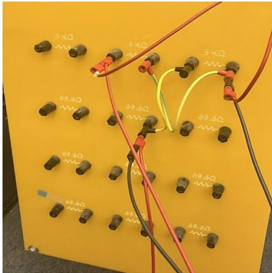
Figure 16: The load used for the battery test WITH two  $5\text{ k}\Omega$  resistors in parallel, a total load of  $2.5\text{ k}\Omega$ .
