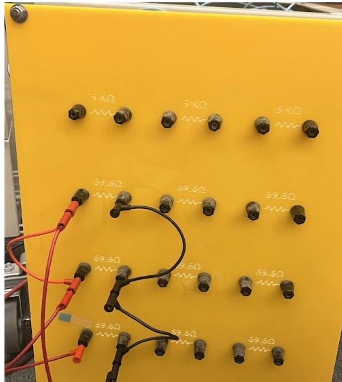
Figure 19: Three parallel  $69.6\text{-}\Omega$  resistors load configuration equal to  $23.2\text{ ohms}$ .
