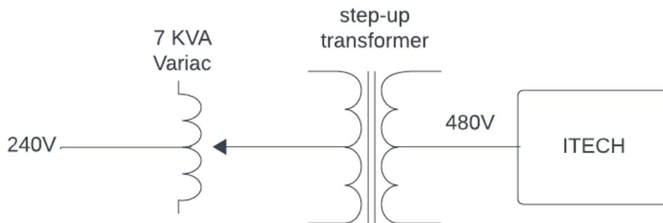
Figure 10: ITECH supply wiring diagram
