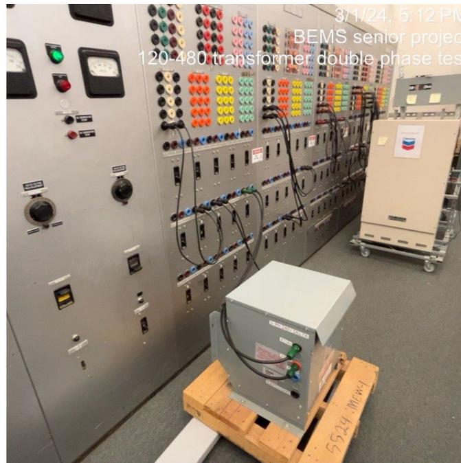
*Figure 7: Step-up transformer during open circuit test*
