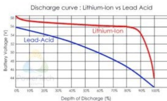
Figure 5. Lead-Acid and Lithium-Ion Discharge Rate [8]
