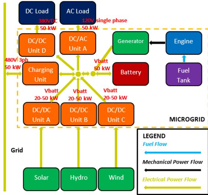
Fig 4. Microgrid Architecture
