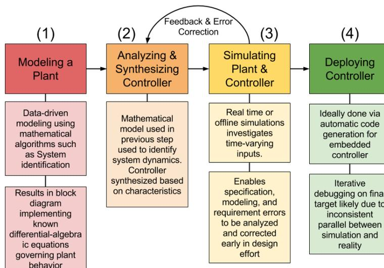
**Fig 1.** Summary of model-based design flow
