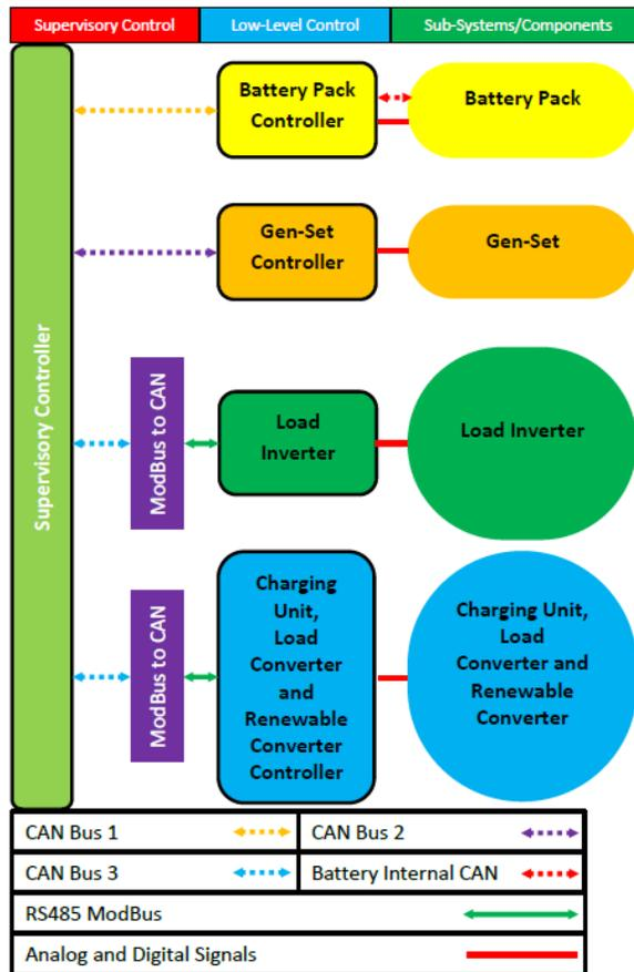
Fig 5. Control system architecture
