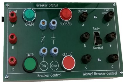
Figure 5. Top View of Final Circuit Breaker
