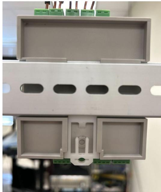
Figure 1 - The OZM V3 GPS mounted to 1.75" DIN rail
