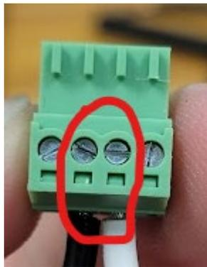
Figure 7 - No strands are touching strands from the other wire, and they are secured to the terminal block.
