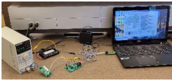
Fig. 3. Testing of the fuel gauge with load bank, battery, and PC software.
