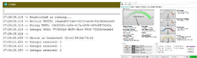
Fig. 8. Serial monitor showing successful BLE communication to app (left). SOC Monitor readings through EVM software (right).
